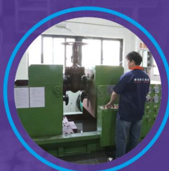
09 检测试压 Pressure Testing
